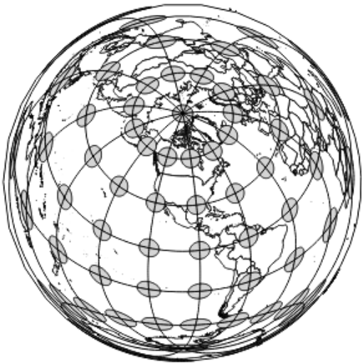
Figure 6. Created caps and graticule on US National Atlas Equal Area projection. (EPSG: 2163, QGIS 2.14.)
