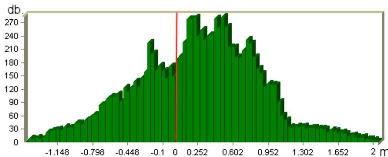
Fig. 5. Function of the differences of the 60m DEM and the 15m DEM datasets
